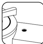
**6.2** If you select pressure level 1, the pressure level indicator will rise to the first mark. When the mark is visible, turn the heat down so that that it remains at this level and no steam comes out.
